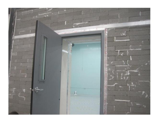
Photo 3. View of receive room from source room through open test specimen #1.
