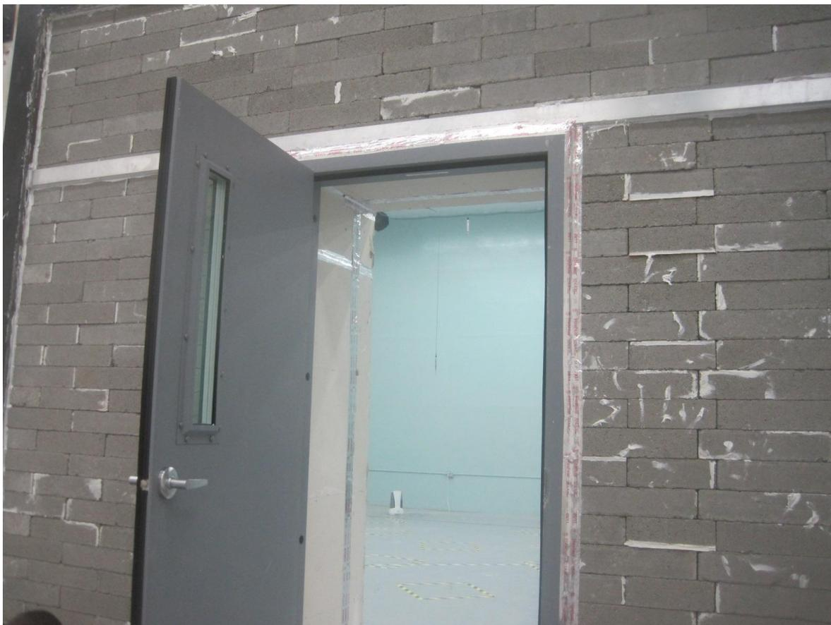
Photo 3. View of receive room from source room through open test specimen #1.
